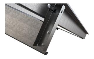
INTEGRATED BONDING Each continuous row is bonded using serrated hardware, therefore only one ground is needed per row. No additional costly grounding components needed such as WEEBS and star washers, lowering material and installation costs. This reduces labor time, hardware, and cost for additional bonding components. (Certified to UL 2703)
